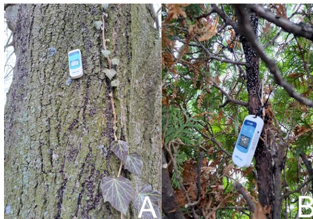
Fig. 1. The temperature automatic data logger: A - inside the thuja shrubs ( T. occidentalis ); B - on the bark of the lime tree at a height of about 2.5 m.
